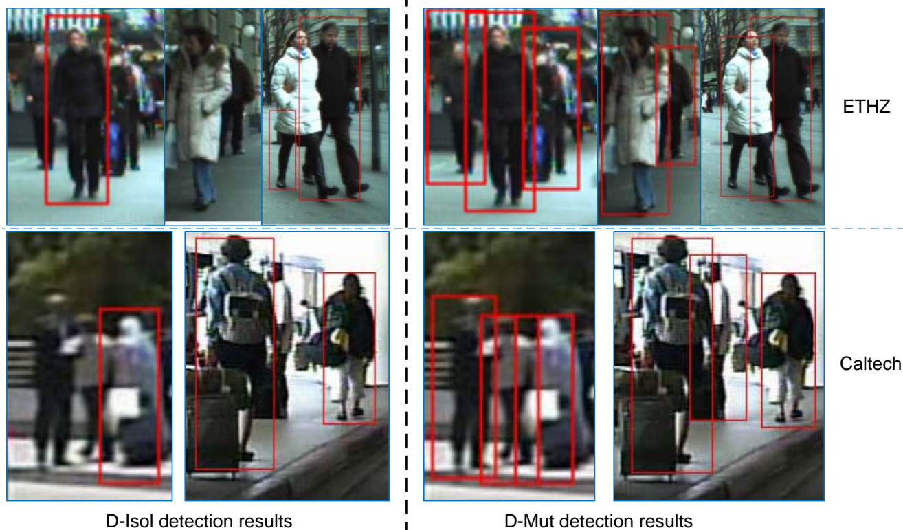
Fig. 7 Detection results comparison of D-Isol and D-Mut on the Caltech-Train dataset and the ETH dataset. All results are obtained at 1 FPPI.
